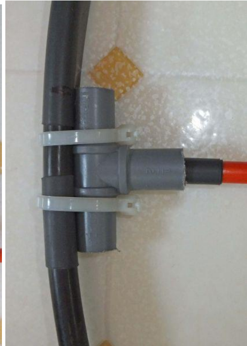
A hose tee with shortened arms is used to secure the loop to the support arm.
